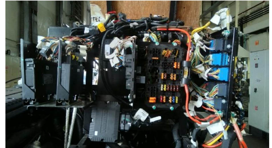
Electronic control unit main cabinet
